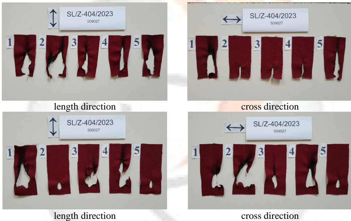
Figure 4. Appearance of the sample after the small burner test
